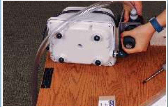
Push the black bulb up and give it a quarter turn to unlatch then pull down
