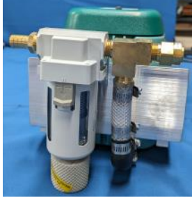
Compressor (s) with filter
