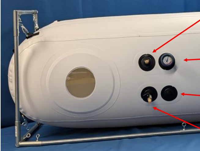
CENTER ARRAY OF VALVES AT HEAD END OF CHAMBER
