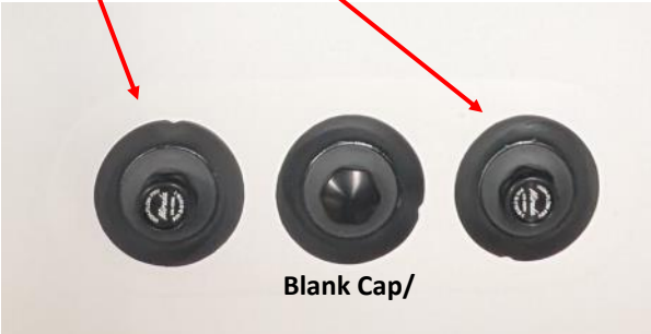
HEAD END VALVES—Note: 27" chamber has only 2 Pressure relief valves at the head end
